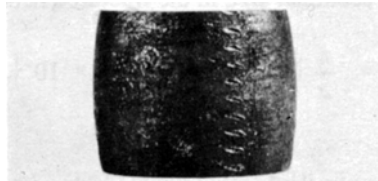
Figure 1.14 Barrel-like failure in a compressed specimen of mild steel.
